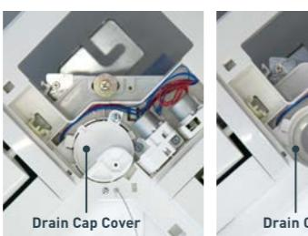
Remove drain cap cover and check the condition. To clean, firstly remove the rubber plug to drain water before removing the drain cap.
