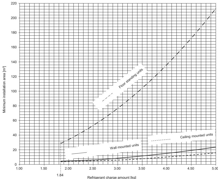
Figure 1. Minimum installation area (A min) graph
