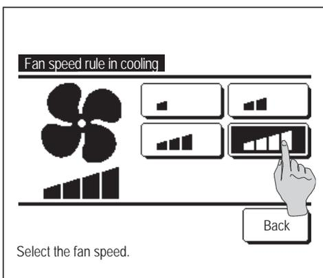
**7** Set the fan speed in cooling mode.
