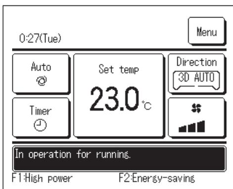
**5** When the 3D auto flow operation is enabled, "3D AUTO" is displayed on the **Change flap direction** button, as shown on the left.
