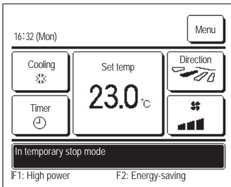
These messages will be displayed when the unit is operated through IO external input.
