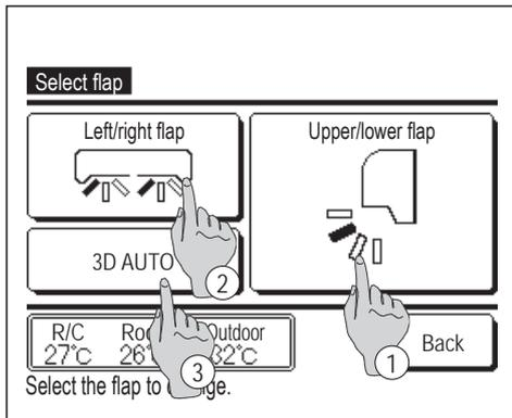
**3** When one or more FDKs with a left/right flap are connected, the Select flap screen is displayed. Select the desired flap direction.
