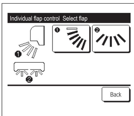
For an FDK with a left/right flap, select the upper/lower flap or left/right flap.
