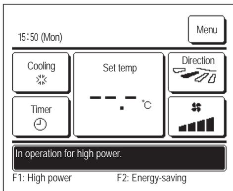
**1** Push the **F1** ( **F2** ) switch to start the high power operation.
