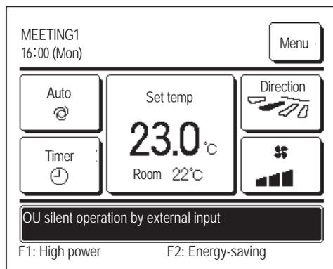
When “OU silent operation by external input” is displayed, the operation performed will be the same as the silent mode control (page 72) performed from the R/C.
