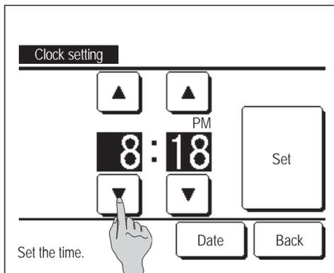
3 Set the "hour : minute" with the   buttons on the clock setting screen.
