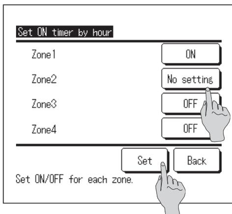
9 Tapping the  button makes it possible to perform zone operation settings at the time of timer working. Set  /  /  (No setting/OPEN/CLOSE) for each zone during timer operation.
