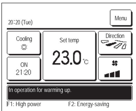
When you select to enable warming up by the Set ON timer by hour (☞ page 44) or Set ON timer by clock (☞ page 47), the operation will start 50 to 60 minutes earlier, which is predicted based on the previous warm up operation, so that the room will be close to the set temp by the time it reaches the operation start time.
