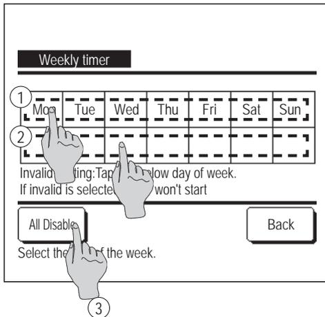
**3** When a desired day of the week ① is tapped on the display, contents of current setting for the day are displayed. (☞5)
