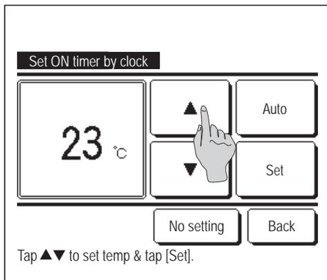
**6** Select a desired temperature (at 1°C intervals) with the ▲ ▼ buttons. Or tap the Auto button and select the auto temp setting.
