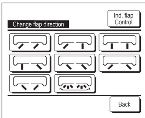
**4** Tap the desired flap direction. After selecting the flap direction, the display returns to the Select flap screen. (➡1)
