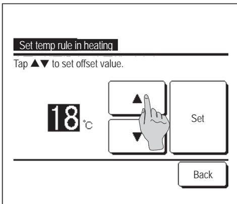
**6** Set the indoor temperature to start operation in heating after setting the “Determine temp rule in heating”.
