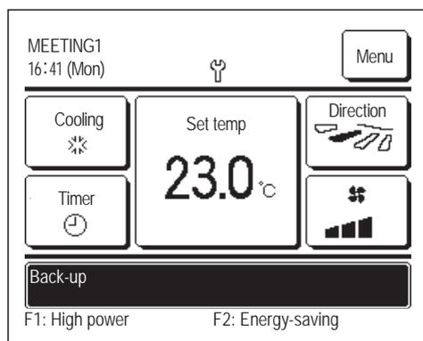
When the “Back-up” is displayed, contact dealer/company shown as the Contact company (page 76) immediately for checking.
