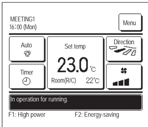
When R/C sensor setting is enabled, the room temperature (R/C)  $\text{°C}$  is displayed (refer to the installation manual on how to make these settings).
