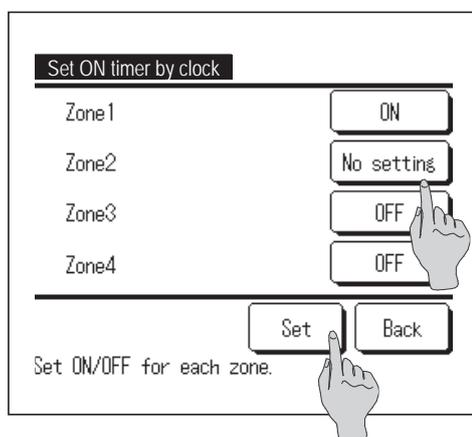
**9** Tapping the Zones button makes it possible to perform zone operation settings during timer operation. Set No setting / ON / OFF (No setting/ OPEN/CLOSE) for each zone at the time of timer working.
