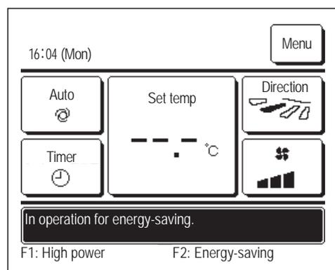
**1** Push the **F1** ( **F2** ) switch to start the energy-saving operation.
