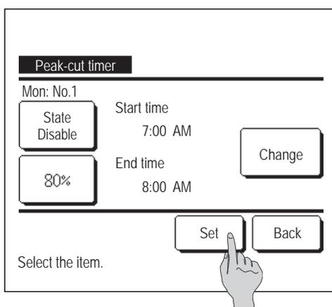
**10** The setting content check screen (☞6) is displayed. If the  button is tapped, the contents are confirmed and a day of the week setting content check screen (☞5) is displayed.
