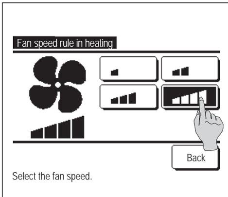
**8** Set the fan speed in heating mode.
