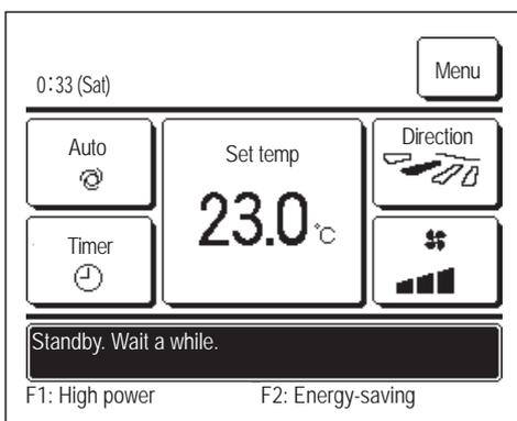
The message “Standby. Wait a while.” may be displayed (maximum of 30 minutes) on the R/C during the first operation following a breaker power on or power loss.
