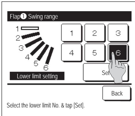
**5** Select one of the lower limit positions from  to  for the flap motion range.
