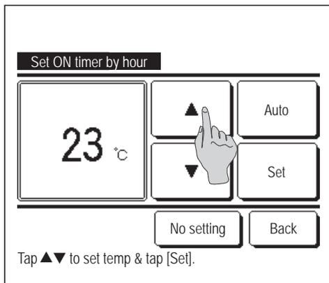
6 Select a desired temperature (at 1°C intervals) with the   buttons. Or tap the  button and select the auto temp setting.
