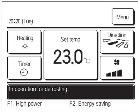
When frost forms on the OU, the heating performance will decrease. This will cause the unit to automatically switch to defrost operation, and hot air will stop blowing out from the IO. The message “In operation for defrosting.” will be displayed on the message display. After the defrost operation has completed, “In operation for defrosting.” will disappear, and the unit will switch back to its normal heating operation.
