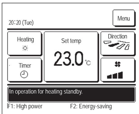
To prevent any cold air blowing out from the IO at the start of a heating operation, the unit stops the fan and displays “In operation for heating standby.” on the message display. When the unit is ready to blow out hot air, the message “In operation for heating standby.” disappears, and the unit will start heating operation.
