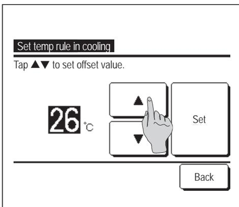
**5** Set the indoor temperature to start operation in cooling after setting the “Determine temp rule in cooling”.
