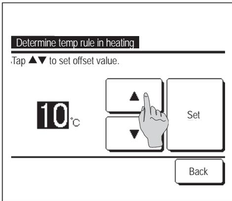
**4** Set the outdoor temperature for the “Determine temp rule in heating”.
