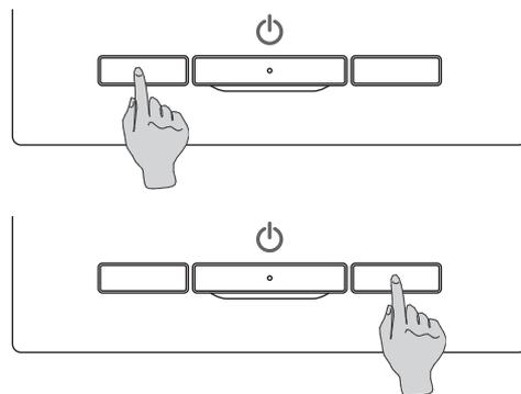
Changing the function of the **F1** or **F2** switch can be performed with the F1/F2 function setting (☞ page 71).
