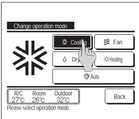
2 When the Change operation mode screen is displayed, tap the button of desired mode.
